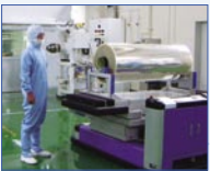
Triacetyl-cellulose (TAC) film for LCD polarizing plates
