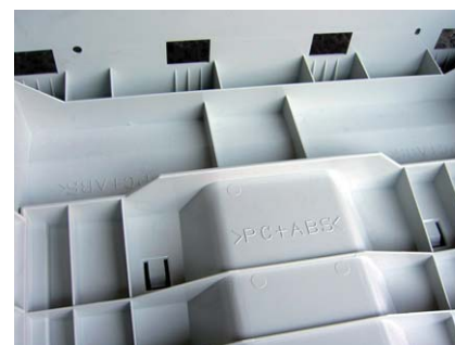
Outer casing parts made of PC-ABS
