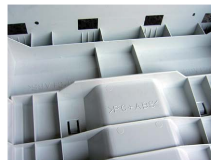
Outer casing parts made of PC-ABS
