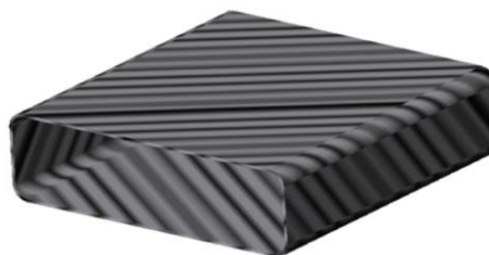
Fig.4 Monocoque-structured carbon chassis.
