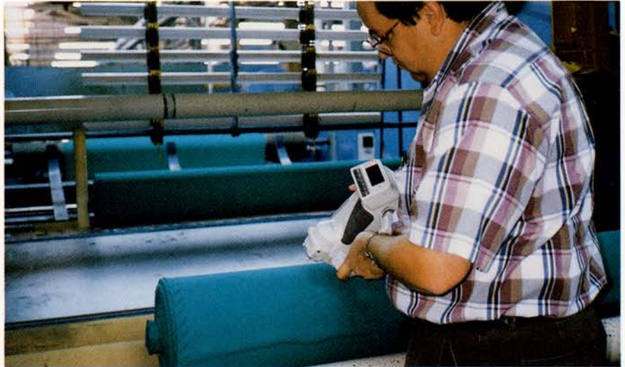
Portable spectrophotometers such as this Minolta CM-2002 enable measuring color directly on the factory floor.
