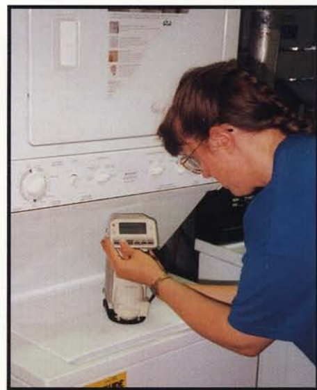
Color is checked on a Frigidaire laundry center with a Minolta CM-503i spectrophotometer.
