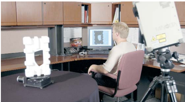
RMKI chose the Konica Minolta VIVID 3-D digitizing scanner as the ideal instrument to turn existing dunnage parts, such as this plastic automotive electronics shipping case, into modern CAD/CAE/CAM software files.
