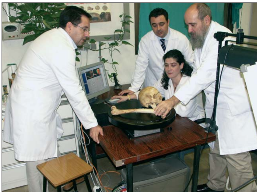
Arrangement of scanning objects on a Konica Minolta rotating stage.
