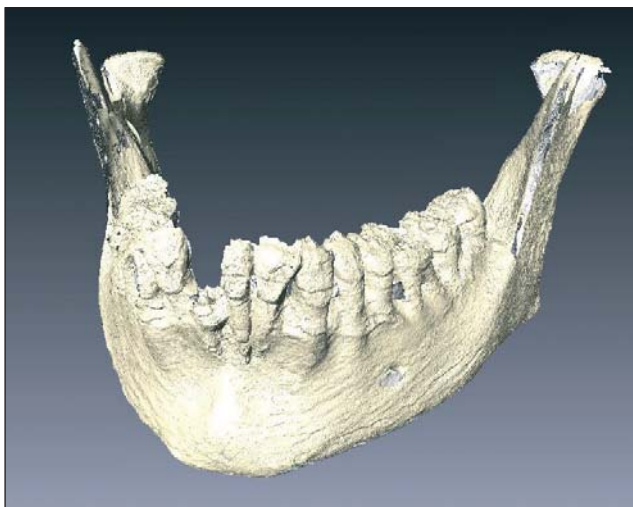
“Raw” output of the VI-910 3D Digitizer. Even the surface of the bone can be recognized.
