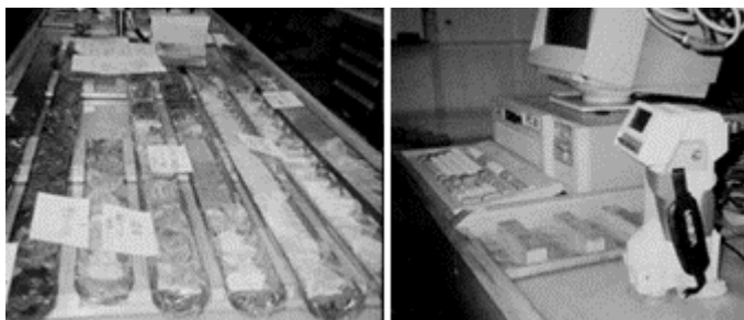
[ Left ] Measurement sample / [ Right ] Spectrophotometer used on board
