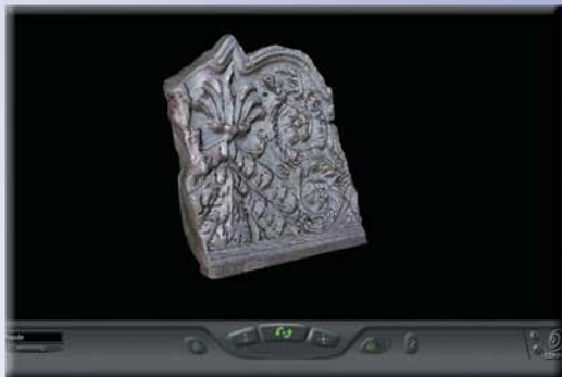
VRML model in 'Cosmo Player'. Zoom step 4, resolution x,y = 1.25mm, res. z = 0.61mm Field of view ca. 25 x 25cm, Total number of scans =34, each shot max.10.000 3D points. Accuracy ±1mm.
