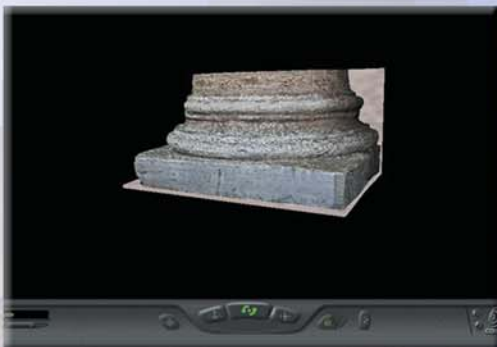
VRML model in 'Cosmo Player'. Zoom step 4, resolution x,y =1.25mm, res. z = 0.61mm. Field of view ca. 25 x 25cm. Total number of scans = 41, each shot max. 10.000 3D points. Accuracy ±1mm.
