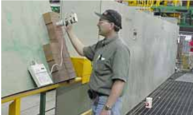
Figure 2: Reading the Color of a Production Run
