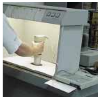
Figure 6: Color Check of a Red Iron Oxide
