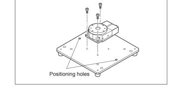
Tighten the three hexagon bolts using the hexagon wrench supplied with the product.
