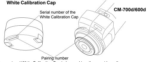
The instrument and White Calibration Cap to be used together must have the same pairing number.
