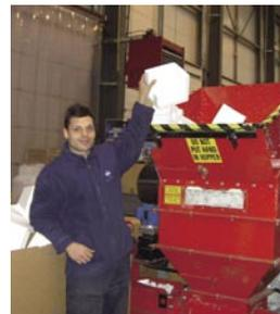
Mechanically compacting waste
