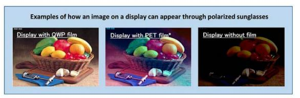
The image of the "Display with PET film" is an example of how an image can appear when PET (polyethylene terephthalate) film is applied on a display in place of QWP film.
