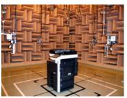
The inside of the acoustic test laboratory
