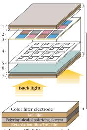
4 sheets of TAC film are required per 1 LCD display
