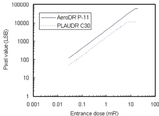
Fig.3 Digital characteristic curves of AeroDR and PLAUDR.
