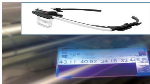
Fig. 9 Realtime data about film making process displayed on smart glass. Operators monitor the process information in real time and operate properly by using the system. It also enables smooth, real-time information sharing among operators in different places, leading to more stable manufacturing process.
