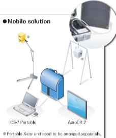
Konica Minolta can offer a mobile DR system with AeroDR 2 1417S for home care, disaster medicine. As system components such as panel, console PC and a access point\*4 and Battery charging unit can be packed in Konica Minolta special designed carrying bag, users can carry the system easily.
