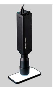
The CA-527 offers industry-leading<sup>\*4</sup> low luminance measurement and high speed. The application function has also been enhanced in line with the technology trend of cutting-edge displays. The product meets the latest evaluation needs of highresolution next-generation displays, such as increasingly higher-dynamic-range (HDR) OLEDs and microLED displays.
