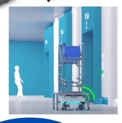
KM also retrofitted 12 automated doors with a wireless communication device which allows the AMR to move without human intervention from room to room.
