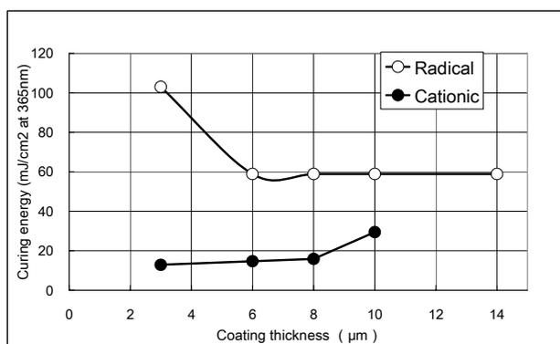
Fig. 3 Effect of coating thickness on curing speed
