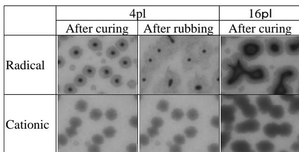
Fig. 5 Optical microscopic images of dots
