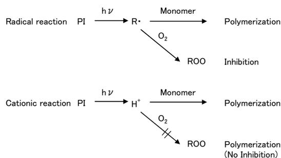
Fig.1 Free radical versus cation polymerization
