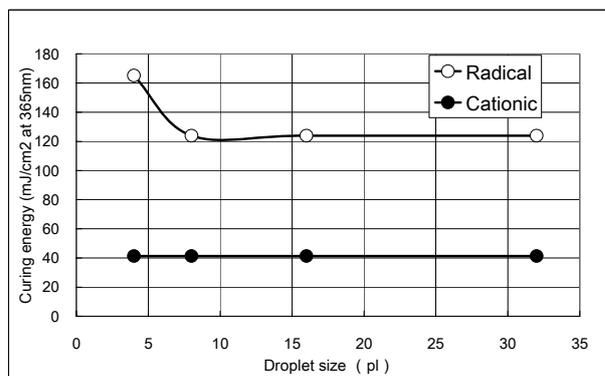
Fig. 4 Effect of droplet size on curing speed
