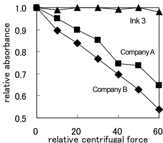
Fig. 7 Sedimentation properties of three inks
