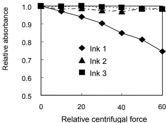
Fig. 1 Sedimentation properties of three inks
