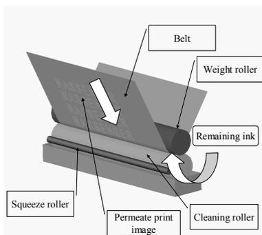
Fig.5 Schematic diagram of the belt cleaning system
