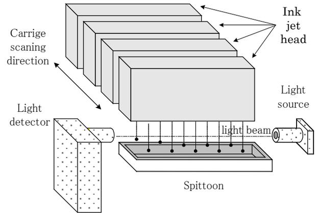
Fig.9 Schematic diagram of ink drop detection system
