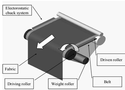
Fig.3 Schematic diagram of the belt feed
