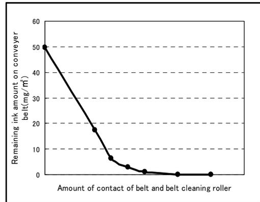
Fig.6 Relation between pressure of the cleaning roller and remaining ink amount on belt
