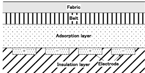
Fig.7 Cross section of adhesion system
