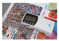
By measuring the environm ental light source with an FD-7 master body and then transferring the user illuminant data to multiple FD-5 or FD-7 working bodies, color cont rol using the same illumination light source at multiple locations can be achieved. In addition, the automatic wavelength compensation function min imizes inter-instrument errors when using multiple instruments.
