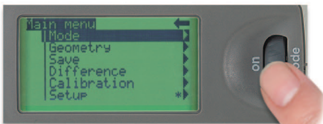
You can select Mode, Geometry selection, Difference, and Calibration from the Main Menu screen.
