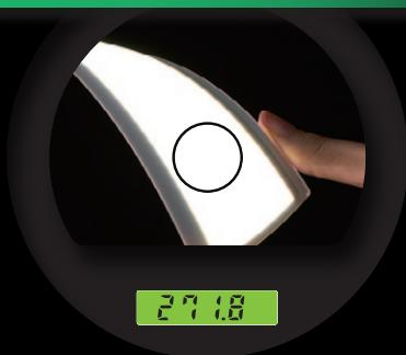
Luminance Meter LS-160 measures luminance from 0.01 to 9,999,000 cd/m<sup>2</sup> with 1/3° measuring angle.
