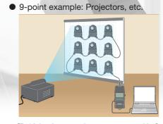
[T-10A 9-point measuring system composition] Illuminant Meter T-10A 1 unit T-10A Receptor head 8 units Adapter units for Main Body T-A20 1 unit Adapter units for Receptor Head T-A21 9 units AC Adapter 1 unit Data Management Software T-S10w 1 set
