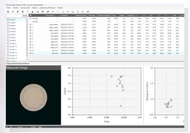
The spectrophotometer must be connected to the CM-SA2 software at the time of measurement to process data and save images.
