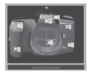
If the scanned data is good enough for alignment processing, the condition bar (under the work window) becomes blue (Good condition), indicating that the conditions are good. If the scan results are not good enough for alignment, the condition bar turns red (No good), indicating that the setup is not good. For the first scan, the bar will be blue if the program successfully detected at least three markers; otherwise the bar will be red.
