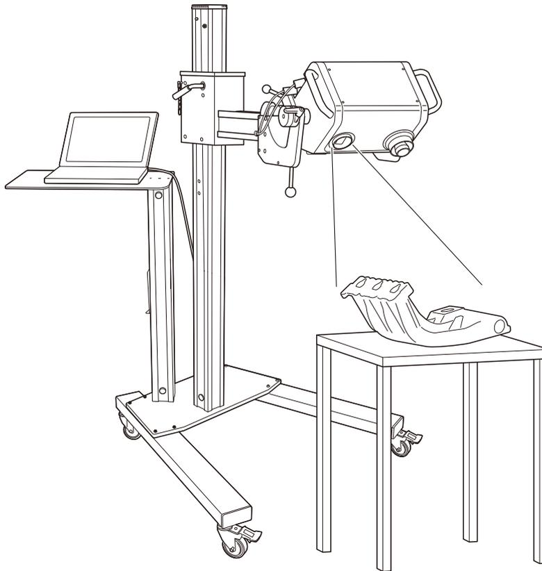
Example of installation on Tripod Set RA-A121 (optional accessory)
