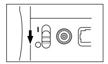
2 Slide the battery cover on the rear of the instrument to open it.
