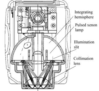
surface of the integrating hemisphere are divided into each wavelength component by the specimenmeasuring sensor and illumination-monitoring sensor respectively. Then, an electric current proportional to the light intensity of each component is output to the analog processing circuit.
