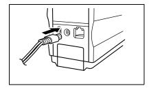
Insert the AC adapter's power plug to an AC outlet (100-240 V AC, 50/60 Hz).
