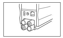
Align the marker on the battery cover with that on the instrument, and slide the battery cover to close it.
