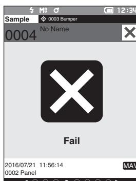
"FAIL" is printed in the print output, and "x" is appended after any value that exceeds the tolerance.
