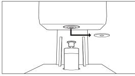
3. Take the desired target mask in your hand, and attach it to the CM-3610A. Make sure that it fits into the concave area around the integrating sphere opening.
