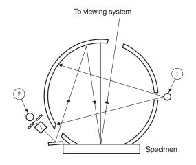
By performing the above measurement and calculation during each measurement, both SCI and SCE measurement data can be obtained simultaneously without the need for mechanical switching.
