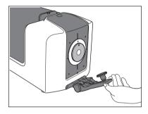
2 As shown in the figure, press on the sample holder so that the sample holder fits into the indentation on the reverse side of the gloss calibration plate.
