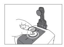
2 Press on the sample holder so that the sample holder fits into the indentation on the reverse side of the white calibration plate.
