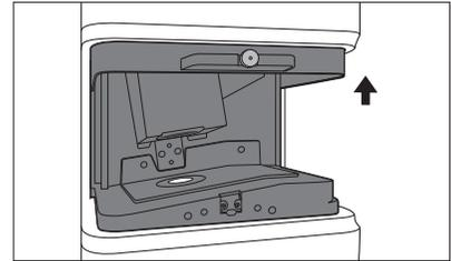
The lock can be released when you want to slide the cover freely. Pull the knob toward you and rotate it 90 degrees to release the lock and free the cover to be opened and closed.
