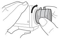
8. Align the threads of the lens and holder, and rotate the outside ring of the holder until it is tight. (Be sure that the tightening screw of the holder is loose.)
