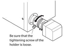
**10**. Tighten up the tightening screw of the holder.
