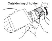
**9.** While the tightening screw of the holder is still loose, rotate the camera while monitoring the shooting screen to align the rotation direction of the camera.
