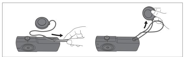
2 Pass the cap through the ring in the cap's strap, and then pull the strap tight to fix the cap in place on the main unit.
