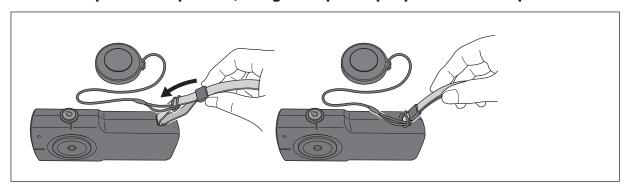
When the instrument is not in use, attach the cap to the light-receiving window as shown in the following figure.
