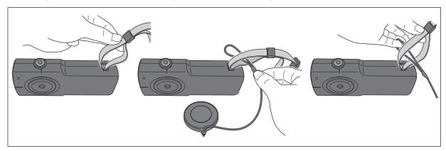
**5** Pass the cap through the ring in the cap's strap, and then tighten the knot in the strap.
