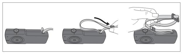
Pass the wrist strap through the buckle, adjust the length of the wrist strap, and then fix it in place.
