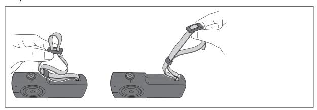
If you will only attach the wrist strap, proceed to step **6** and slide the loop to the strap holder, fixing the strap in place on the strap.
