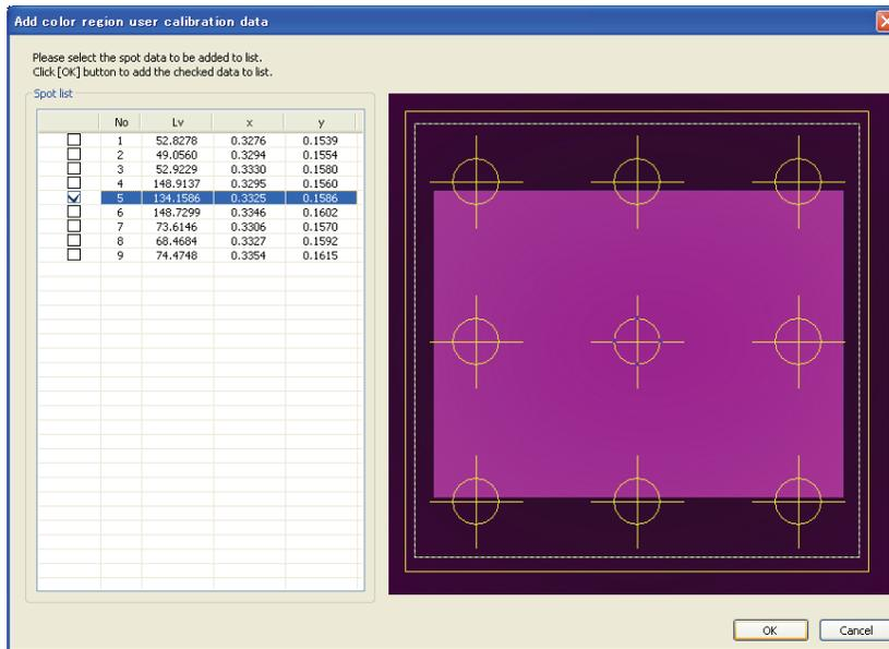
When you select spot data used for calibration data from the list and click the OK button, calibration data is added to the list of the Create color region user calibration file dialog box.
