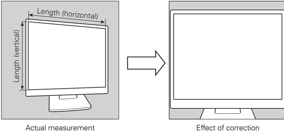
In addition, there are cases where the measurement target is displayed in an inclined manner due to the misalignment of installation between the measurement target and the CA-2500/CA-2000. When this option is selected, the image can be corrected so that the measurement target and the display screen of the CA-2500/CA-2000 are parallel in the vertical and horizontal directions.
