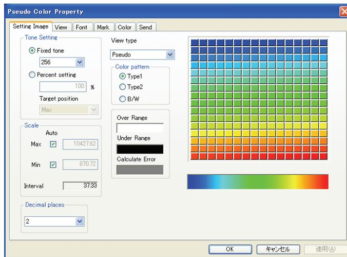
When ‘Auto’ is checked, the measurement data’s maximum and minimum values are used.
