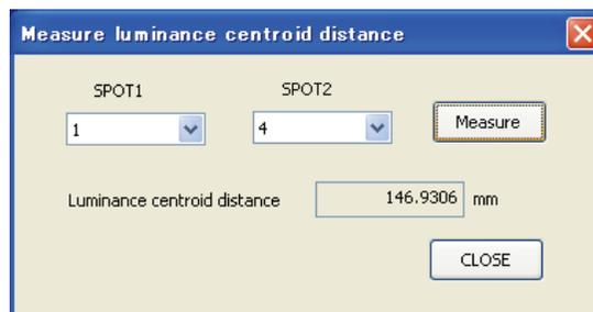
3. Select two spot measurement frames for which the distance between the luminance centroids are to be measured and click 'Measure' button.
