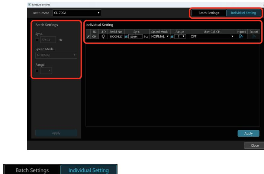
**Batch Settings:** These settings are applied as a batch to all the connected instruments. The items that you can set in this manner are **“Sync.”**, **“Speed Mode”**, and **“Range.”**
