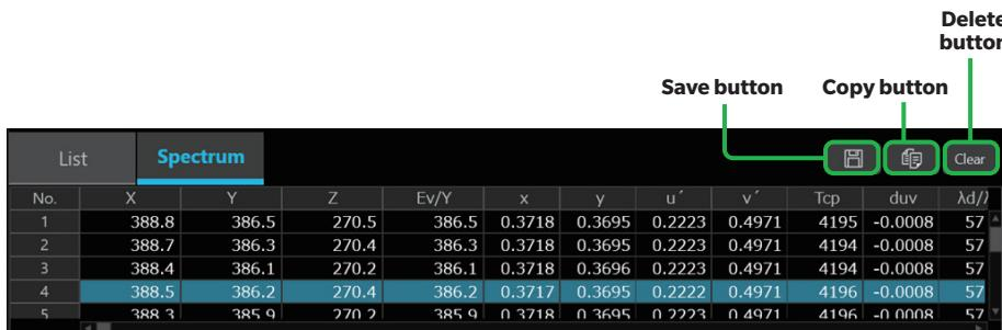
The screenshot shows a measurement data list with the 'Spectrum' tab selected. The data table has columns for No., X, Y, Z, Ev/Y, x, y, u', v', Tcp, duv, and λd/l. The first five rows of data are shown. Above the table is a toolbar with buttons for Save, Copy, and Clear. A green line points from the 'Save button' and 'Copy button' to these toolbar buttons. Another green line points from the 'Delete button' to the 'Delete' button in the toolbar.
