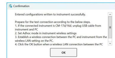
B-9. In the computer's Wi-Fi settings ("Settings" - "Network & Internet" - "Wi-Fi" - "Show available networks" on Windows 11), select the instrument's SSID, click the "Connect" button, and input the Authentication Key input in Step 2-② when requested.
