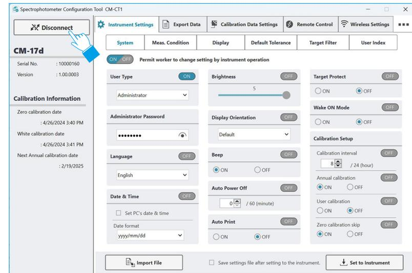
Clicking the "Disconnect" button will end communication with the spectrophotometer, and the screen will return to the dialog for connecting to a device.
