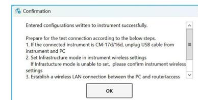
B-11. Connection between the computer and instrument via the specified access point will be tested, and if successful the message box at right will appear.
