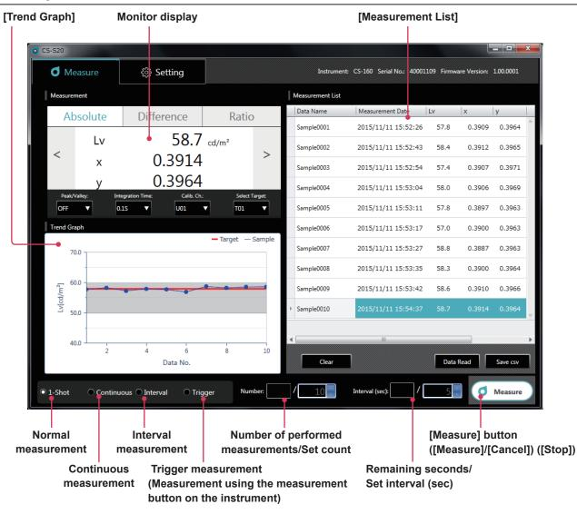
Normal measurement, continuous measurement, interval measurement, and trigger measurement
