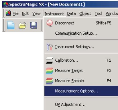
2. Specify the parameters for the auto-averaging measurement and calibration interval.
