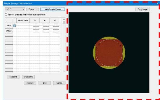
When the CM-36dG, CM-36dGV, or CM-36d is connected, the Sample Viewer panel (indicated by red dotted-line rectangle above) will be shown when Show Sample Viewer has been clicked.
