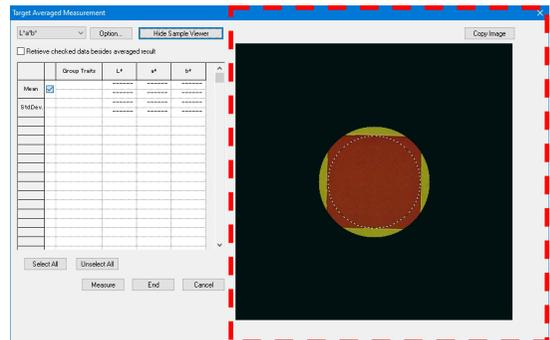
When the CM-36dG, CM-36dGV, or CM-36d is connected, the Sample Viewer panel (indicated by red dotted-line rectangle above) will be shown when Show Sample Viewer has been clicked.
