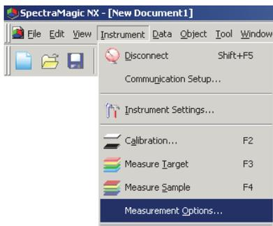
The interval measurement repeats measurement a specified number of times at specified intervals. The measured sample data is received after every measurement.
