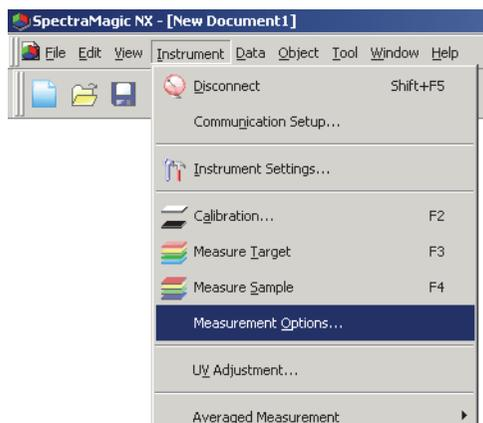
During automatic averaging measurement of sample data, measurements are repeated the specified number of times. When the measurement is completed, the collected sample data is averaged to obtain one piece of sample data.
