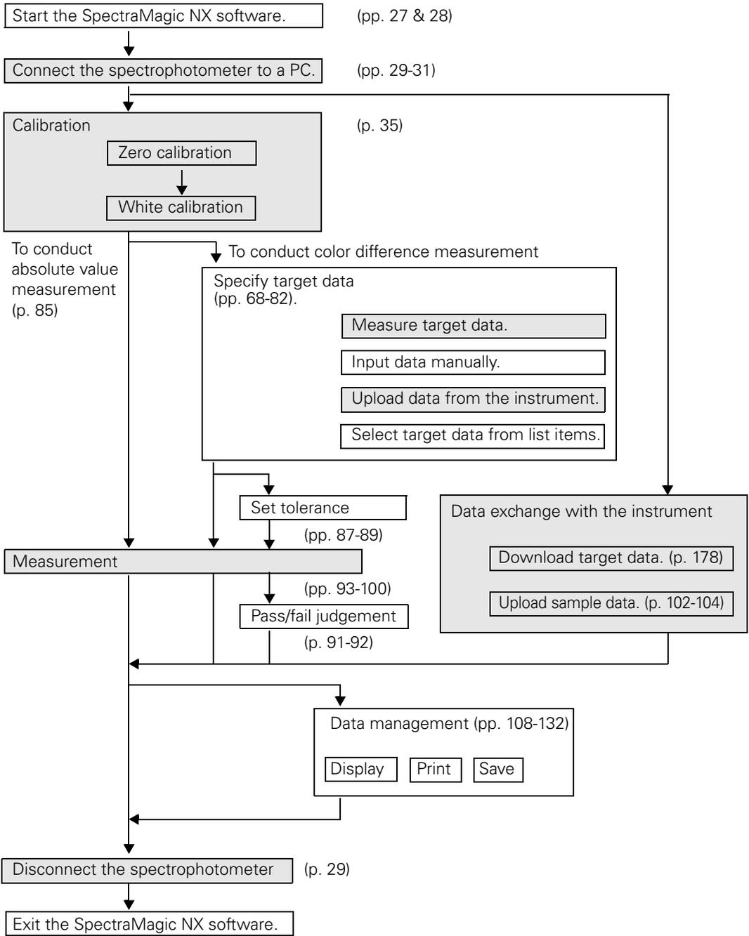
The shaded sections indicate functions available only when the spectrophotometer is connected and the protection key is attached to the computer.
