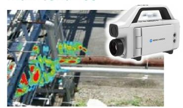
Immediate measurement of gas leakage location and flow rate
