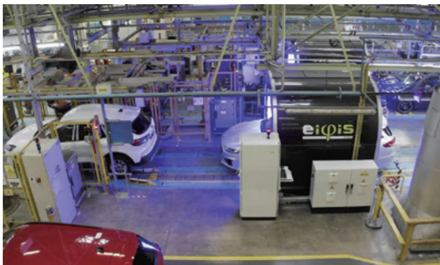
Eines' automated quality inspection system for automobile production
