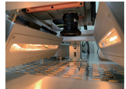
Quality test of pharmaceutical products using HSI camera
