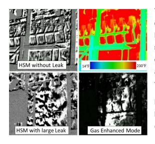
This is a prime example of how altering the sensitivity level really does the trick in clarifying an image. Once the heat saturation has been removed, the noise from the heat can be confirmed on the surface of high heated parts, which causes interference with the gas plume in the HSM. The Gas Enhanced mode assists with this aspect, and makes the emissions brighter and more visible then the surrounding background.
