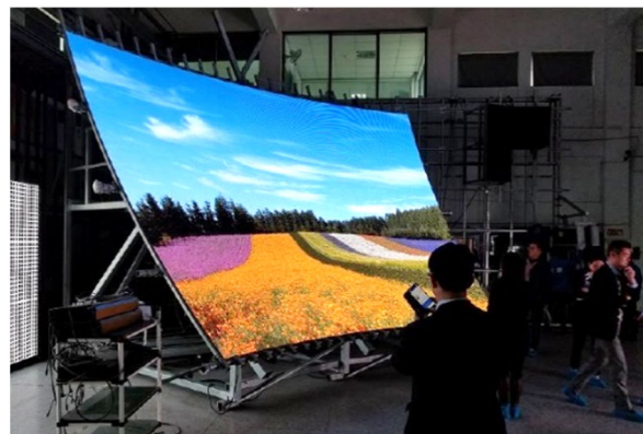
Panel of the LED dome system in part
